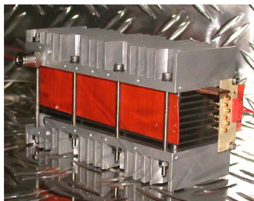
Fig. 7. Outdoor fuel-cell stack with internal humidifier, electric heating, cooling ribs and single-cell contact pins for monitoring.
